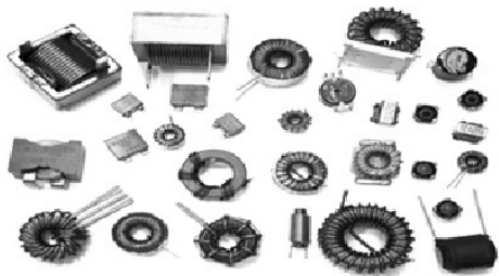
Fig. P7.4: Image showing various types of inductors
