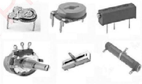
Fig. P7.2: Image showing various types of variable resistors (Courtesy:Technicalegg)
