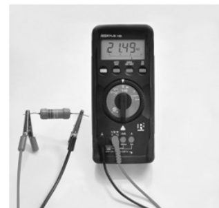
Fig. P13.2: Resistance Measurement using Digital multimeter
