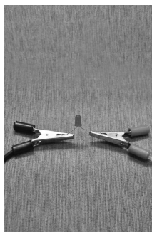
Fig. P17.2: Image showing crocodile probes connected to LED
