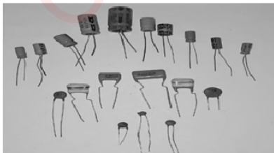
Fig. P7.3: Image showing various types of capacitors
